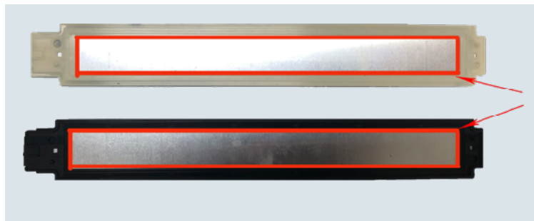
PTC heater electric heater : Plastic housing and aluminum interface adhesion
